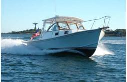
spray rails are employed when the hull has a particular issue with excessive "wetting".
