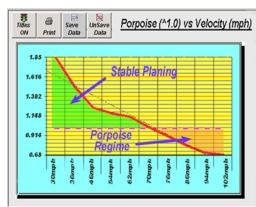
We have developed a new analysis tool in the TBDP©/VBDP© software that helps predict your hull's inherent instabilities leading to porpoising. The technique is a prediction of the critical porpoise trim angle (CPA) and shows the velocity at which your hull configuration will experience instability in Porpoise Regime and has a susceptibility to porpoising.
