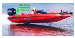
Lift (CofL) as the boat accelerates. The relocation of static weights is one way of dampening the rate of change of the CofL...so it's not always obvious whether to move weight fore or aft in order to cause the "dampening". The solution can be calculated, but it's also not too difficult for you to test by moving weight fore or aft, to help your particular problem.
