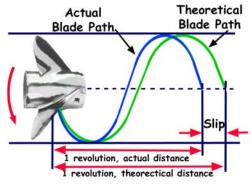
'Prop Slip' is not a measure of performance, but rather a calculation that helps compare the performance of different propeller setups on a hull. Slip is the difference between the propeller's actual distance travelled and the theoretical distance of travel.
