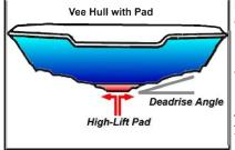
hydrodynamics dictates that a steeper angle of Vee (for example 20 degrees) or "deadrise", creates less Lift than a shallow angle of Vee (say, 10 degrees). The extreme case of the completely flat Pad that has a zero (0 degrees) deadrise creates very high Lift for it's small wetted surface area. The result of this "extra Lift" is a dramatically reduced hydrodynamic Drag. Less Drag means more speed!
