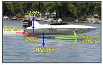
The deeper "V-bottom" boat is the most common of present-day performance Vee hull designs. This design offers a good ride in rough water as the "V-shaped" bottom softens the up-and-down movement (pounding, rough ride in heavy waves). The degree of the angle of the "V" is called "deadrise."
