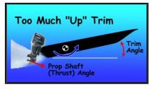
When comfortable at initial acceleration, go to planing speed, progressively trimming UP (out). This will lift some more of the hull off the water, reducing drag and increasing speed. In calm water, you may notice that steering goes light as speed increases with more UP trim. With experience you will note these subtle changes easily in your hull's behavior. If you keep on trimming UP, the propeller may eventually reach an angle where it loses grip, RPMs climb and speed decreases. This can
