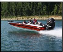
Most outboards and stern drives now include a "power trim/tilt" feature that can change the angle of the engine (or drive unit) and propeller on the transom. Adjusting the running position of the engine/drive is called "trim adjustment", and can easily change the running attitude of the hull. Running at the best "trim" angle can improve fuel economy, increase speed, improve ride comfort, and maintain safe operation of your hull.
