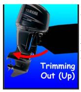
hull, increases top speed, allows more clearance in shallow waters, can cause initiation of porpoising, can cause 'harder' ride in rougher waves
