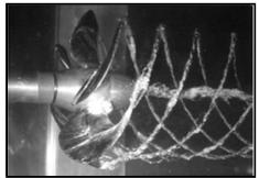
Most all high-performance boaters have experienced the circumstance that restricts their maximum velocity to less than it could be, even though they've got the horsepower available to use. This phenomenon is commonly called "gearcase blowout" or "propeller blowout".
