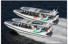
Hobart Cruises has put into service two brand new coastal expedition vessels, each both powered by four Yamaha V8 350hp outboards on the transom. With 1400 hp installed to these two identical 4m aluminium RIB's, Hobart Cruises has established a new benchmark for the burgeoning ecotourism industry.
