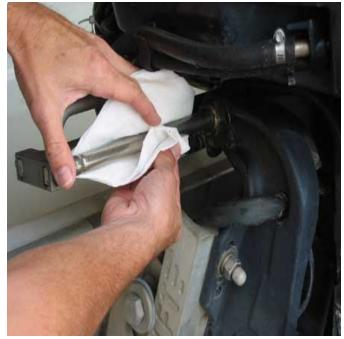
Inspect steering systems, including tiller steering friction fittings on outboards. Tighten them if they're loose. Grease the cylinders on mechanical steering connections to the motor.
