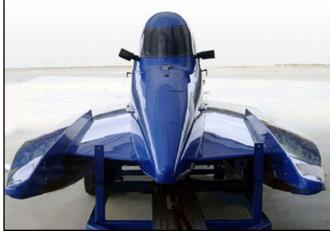
running weight (loaded, including 700 lb of fuel) could be about 7700 lb, and it would have a top speed of say, 105 mph. By running with only 200 lbs less weight (this is only about 2.5 percent less weight) the top speed would increase by 1.5 mph. This may not seem like allot, but remember - the winning boat need only cross the finish line 1 foot sooner than the 2nd place boat! Over a 5-mile racecourse, this represents an advantage for the lighter boat of over a second (or 175 feet) on each lap!
