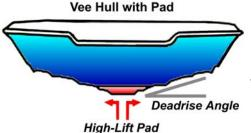
software. We have developed a unique analysis technique that allows designers to see the delicate balance between lift/drag forces of a vee-pad hull. The method allows us to isolate the lift/drag forces for vee-pad, vee (bottom) surfaces, aerodynamic surfaces and lower-unit appendages. This distinctive approach gives the opportunity for designers, builders, owners and operators to optimize the vee-pad dimensions and orientation
