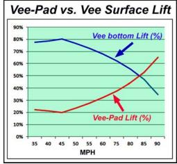
High Lift - The flat pad generates much more efficient Lift than the vee'd bottom shape. Hydrodynamic theory dictates that, in general, a steeper angle of vee (e.g. 20° deadrise)creates less Lift than a shallow angle (e.g. 10° deadrise). The extreme case is the completely flat pad that has zero (0° deadrise) that creates very high Lift for it's small wetted surface area. The result of this "extra Lift" is a dramatically reduced hydrodynamic Drag and more speed!
