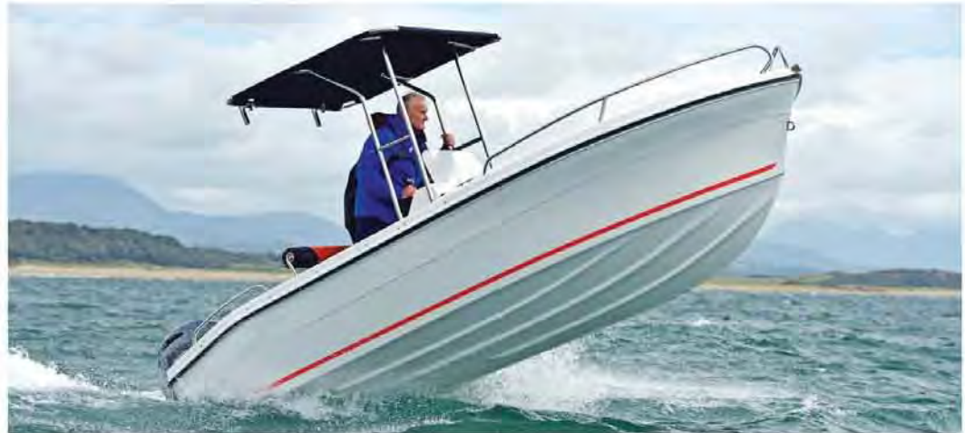
Above: A porpoising boat can be hard to steer.
