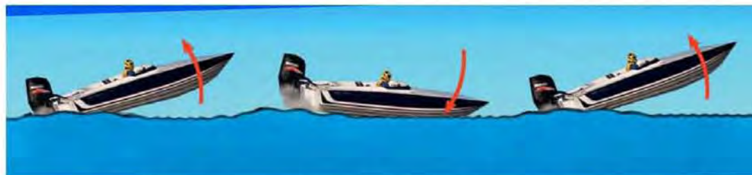
Figure 2: Porpoising is the cyclic oscillation of a boat in pitch and heave with sustained or increasing amplitude.
