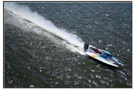
Propeller shaft depth and thrust (trim) angle can affect the efficiency of your propeller thrust, and is often illustrated in how much of a rooster tail you see. Propeller design features also have an affect on thrust efficiency and thus, on the view of the rooster tail. Generally, however, the more "rooster tail" we see, the more INefficient is the trust.
