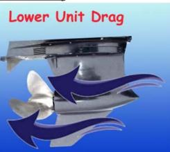
The water density has an effect on the drag of the lower unit too...more dense salt water causes more drag on lower unit. Sometimes this can make as much or more difference as the other contributors! The profile and the exposed drag surfaces of the lower unit remain the same whether it's in fresh water or salt water, so the only difference is the higher density of salt water, so the lower unit drag in salt water is always more than in fresh water.
