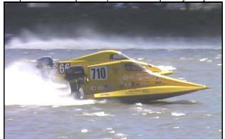
also has the benefit of being able to operate at a reduced (trim) angle of attack (2.9 degrees instead of 2.2 degrees - 25% less), improving the dynamic balance of the hull and even a reduced tendency for porpoising at intermediate speeds.
